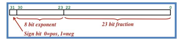
How can we interpret the 32 bits representing a floating point number in single precision?
