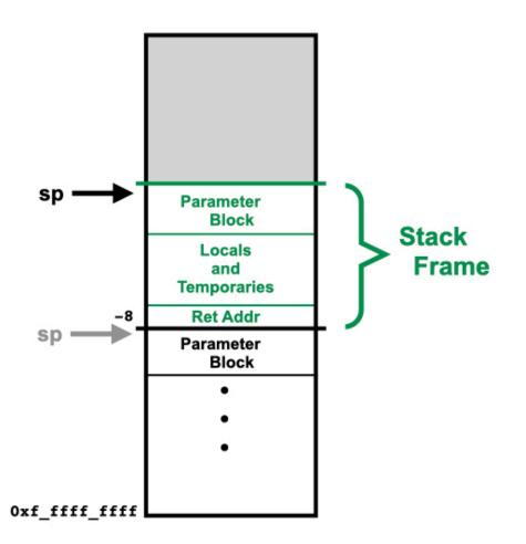
Within foo, the local and temporary variables will be accessed with positive offsets from **sp**. Access to the arguments to foo will also be made using positive offsets to **sp**. The exact offsets to the arguments can only be determined after the size of foo's frame has been determined.
