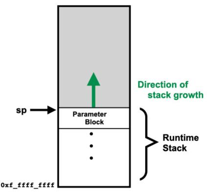
The parameter block will include space for both arguments that are passed in registers and for arguments that must be passed on the stack. For arguments that are not passed in registers, the values will be placed in the parameter block by the caller.
